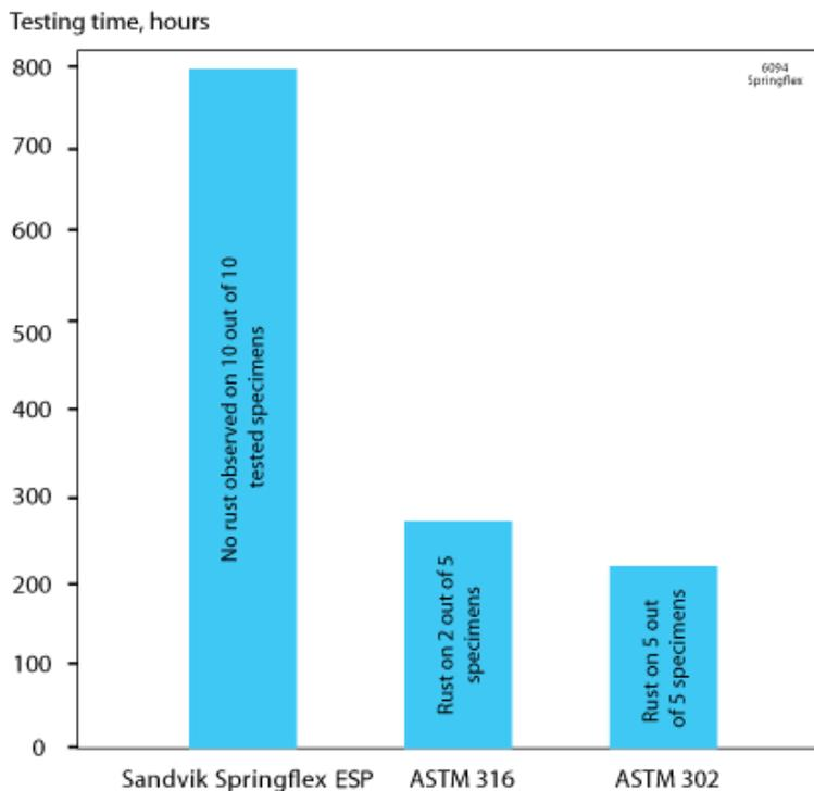
Figure 7. Neutral salt spray test according to ASTM B 117. Springs in the tempered and unpassivated condition were sprayed with neutral, 5 % by volume, salt solution at 35°C (95°F), pH 6.5 - 7.2. Inspections were carried out every 24 hours.
