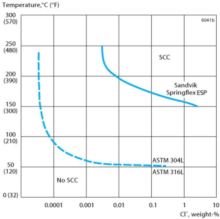
Figure 8. Resistance to stress corrosion cracking, laboratory results for annealed UNS S31803 (Sandvik Springflex ESP) of constant load specimens loaded to 85% of the proof strength at the test temperature.
