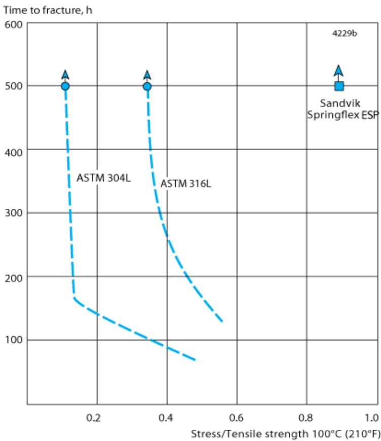
Figure 9. Results of stress corrosion cracking tests on annealed UNS S31803 (Sandvik Springflex ESP), ASTM 302/304L and ASTM 316L in 40 % CaCl<sub>2</sub> at 100°C (210°F) with an aerated test solution.
