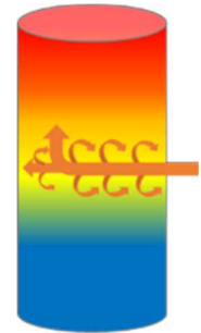
Figure 3 – Inlet jet Mixing
